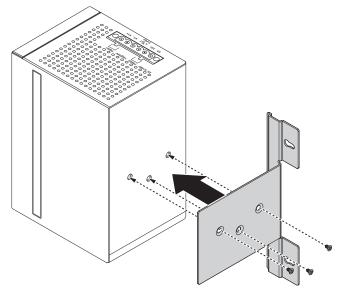
Figure 2.3 Installing Wall Mount Plates
