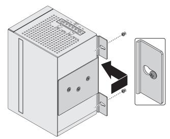
Figure 2.5 Wall Mount Installation
