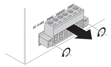
Figure 2.16 Removing a Terminal Block
