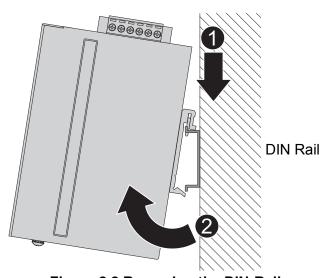
Figure 2.2 Removing the DIN-Rail
