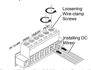
Figure 2.17 Installing DC Wires in a Terminal Block
