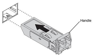
Figure 2.7 Installing an SFP Transceiver
