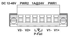
Figure 2.14 Terminal Receptor: Relay Contact
