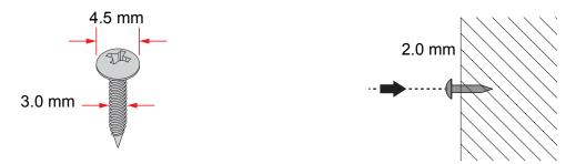
Figure 2.4 Securing Wall Mounting Screws
