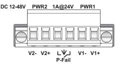
Figure 2.15 Terminal Receptor: Power Input Contacts
