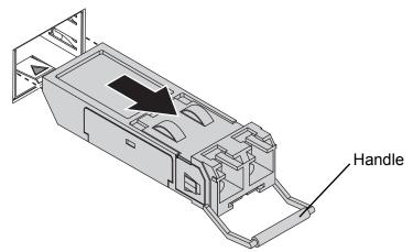
Figure 2.10 Removing an SFP Transceiver
