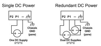
Figure 2.12 Power Wiring for EKI-5000 Series
