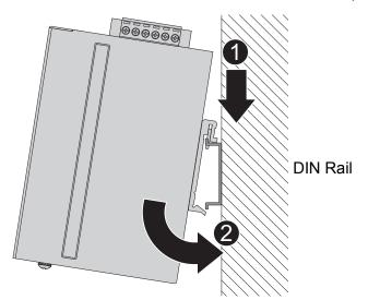
Figure 2.1 Installing the DIN-Rail Mounting Kit
