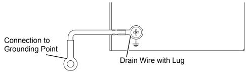
Figure 2.13 Grounding Connection
